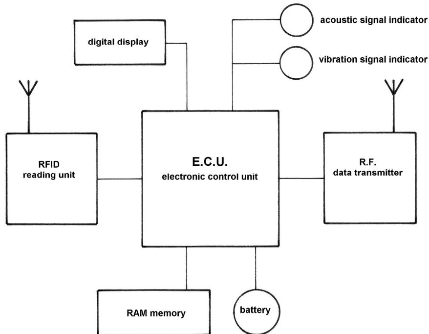
The control unit is a generic one, that is, it is the same for each and all the walkers, as the identification is placed in the sneakers, and not in the control unit, which simply has a self-learning function when it is associated to a pair of insoles. This is extremely interesting for the manufacturing and purchasing cost, because the “expensive” element (control unit) is always reusable, whereas the element that may be replaced and damaged (insoles) is cost-effective.
